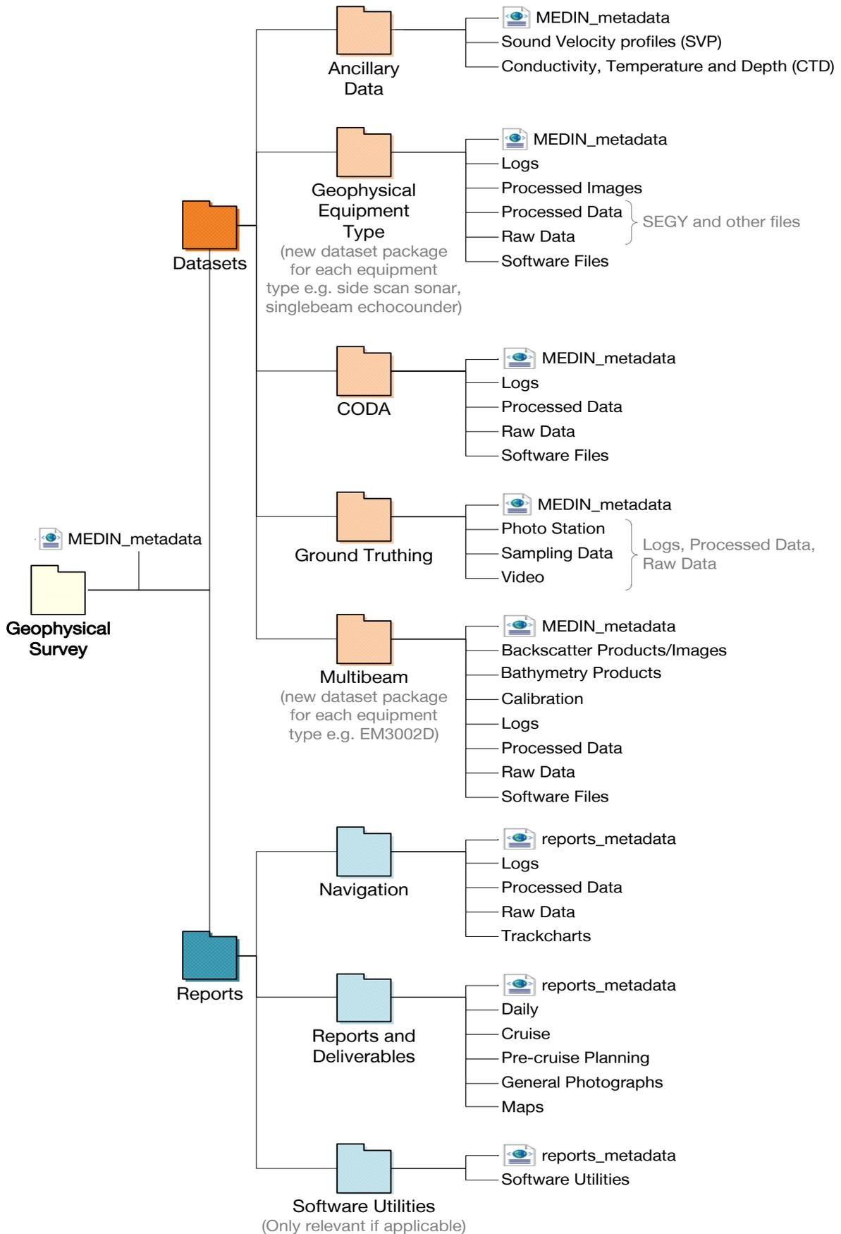
Figure 1 - Example geophysical survey data structure
