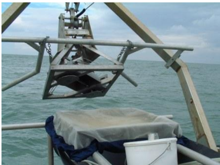
Plate 2. The Day grab aboard the Aquadynamic
