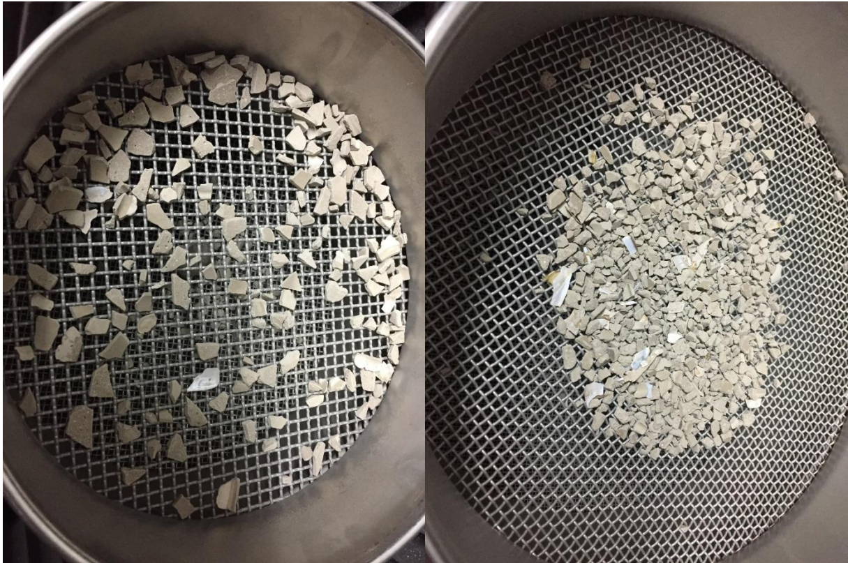
Plate 8 Dried aggregations of mud as a result of pre-drying fine sediments before dry sieving.
