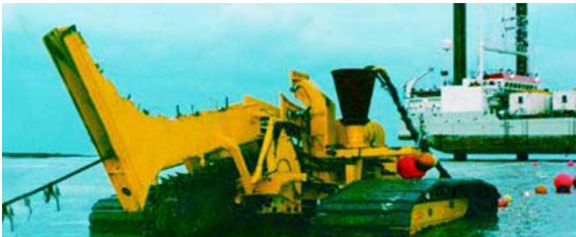
Figure 10 ROV Used for Inter-turbine cable burial (courtesy Global Marine Systems)
